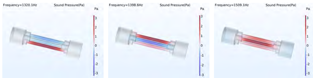
Fig. 1 Simulation of the acoustic pressure in the three resonant cavities at different frequencies.
