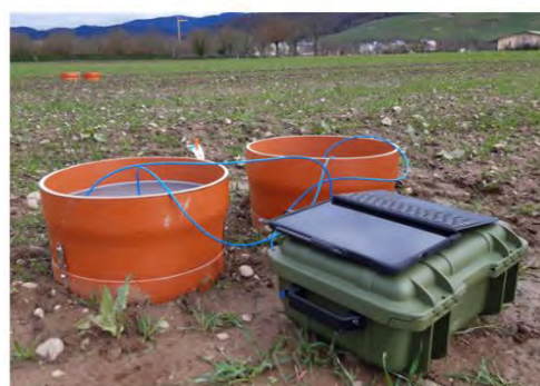
Fig. 1 Schematic setup of the gas circuit in the measuring case including PAS and humidification system (left). Measuring system and N 2 O sampling hoods in the field test (right).
