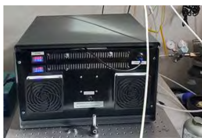
Fig. 1 QEPAS CO 2 analyser prototype and first results at demo site
